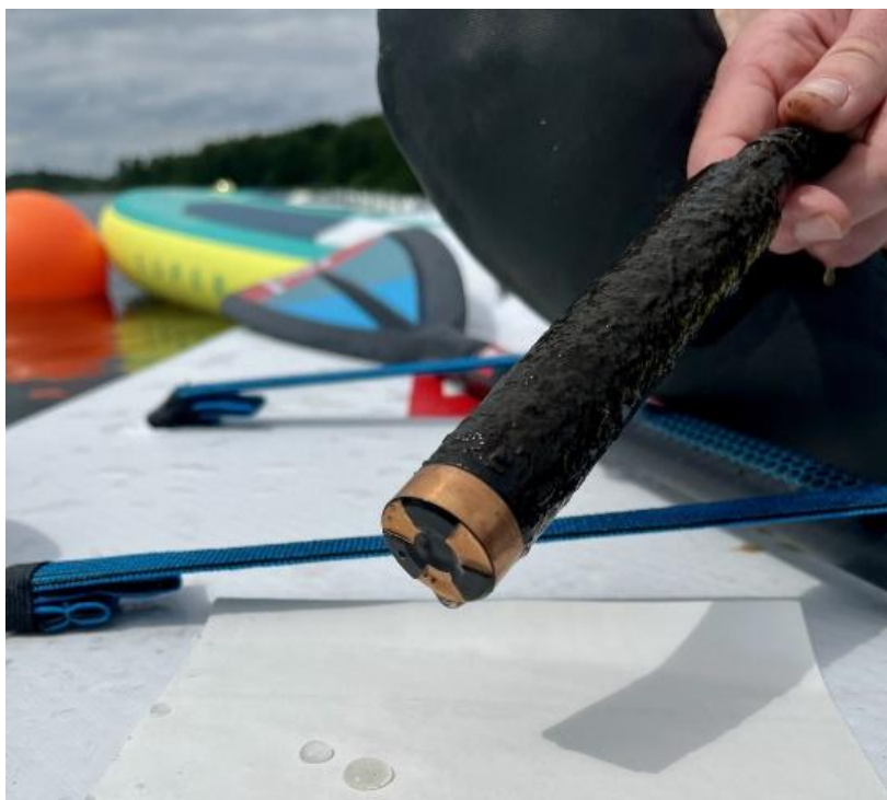
Fig. 1. Example of an OPTOD optical oxygen and temperature sensor, which can be installed in a stream station.
